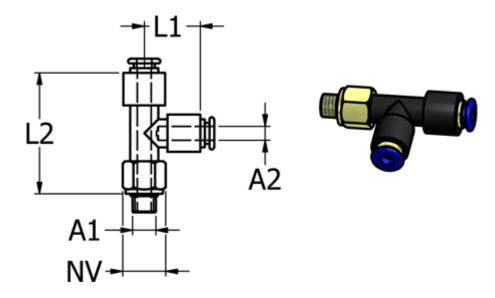
Ext. hose diameter A2 = 3 mm L1 = 12 L2 = 28 NV = 8 Thread A1 = M3
